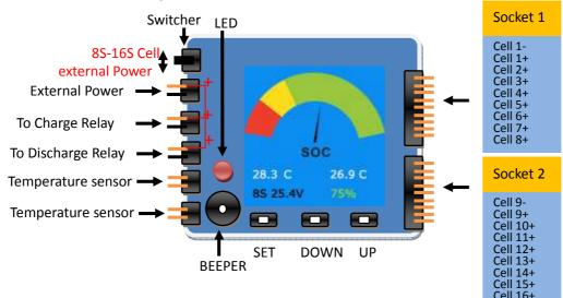
When the switcher is on the external power position, the external Power (VCC) will power the system and the relay coil, as indicated above drawing. The voltage of external power ranges from 15-30V. When the switcher is on the 8S-16S cell position, the system will draw current from all cells and the current is less than 0.1mA even the LCD back-light ON.
