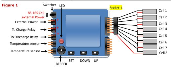
2. For two battery packs, connect them in series first and then plug battery 1# into socket 1, and battery 2# into socket 2 separately. Take one 8S battery and one 4S sample as following:
