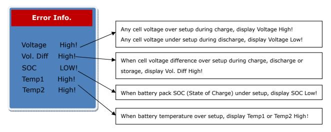
At the same time Alarm port will output the presetting signal ON or OFF. Alarm output port signal ON means the collector connected to Ground. Alarm output port signal OFF means the collector open.
